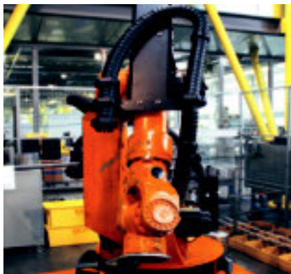
Integrated recuperating spring prevents loop formations
