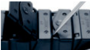
To open Series 352 and Series 353 only - Insert screwdriver into slot on top of lid and push down
