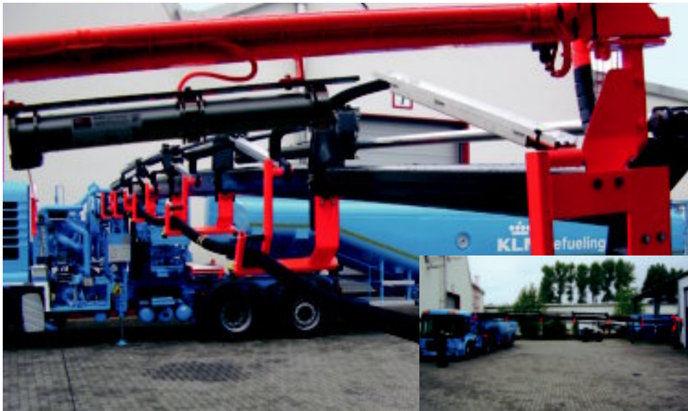
E2/000 Series 1400 in aircraft refuelling truck; telescopic crane with six sections
