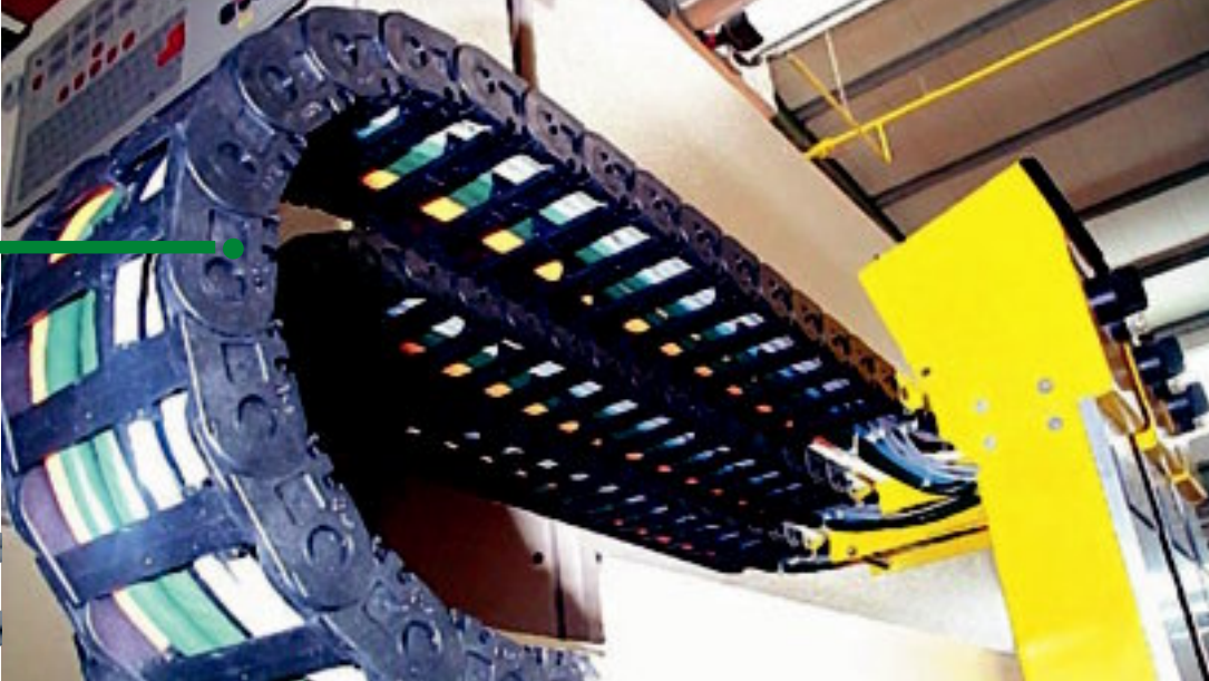
Harnessed E2/000 e-chain® - turnkey solution delivered with cables and sheet metal parts directly to the machine
